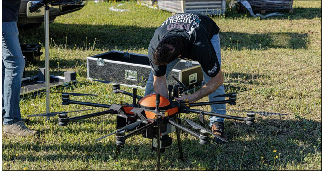
Drone used for digitisation campaigns in Italy and Croatia to take aerial photos and create 'photospheres'
